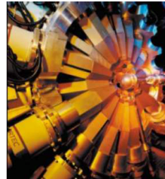
GAMMASPHERE is one of the forefront instruments available for experiments at ATLAS. It consists of 110 Compton-suppressed Ge detectors used to detect gamma rays emitted from compound nuclei formed by fusion of accelerated heavy ions and target nuclei.
