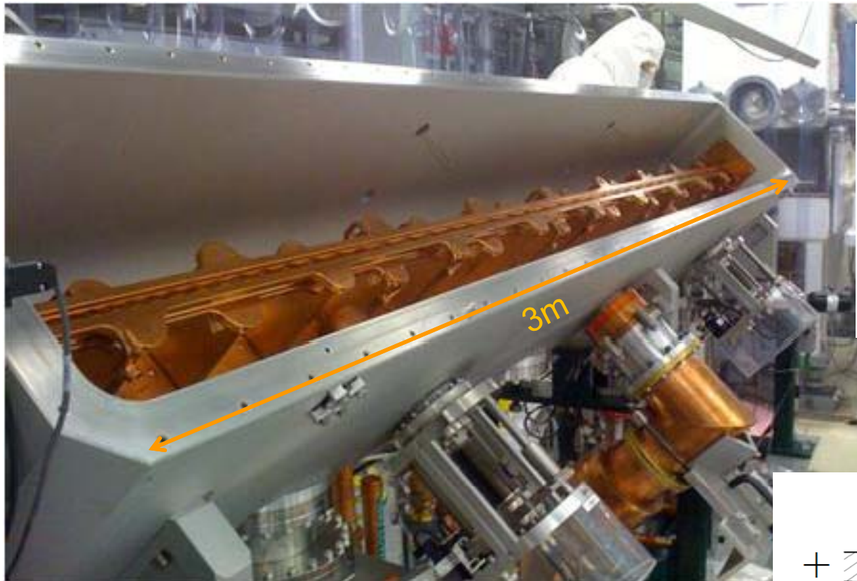
92 cells acceleration cells ReA RFQ accelerator at MSU, energy gain 12keV/u to 600keV/u
